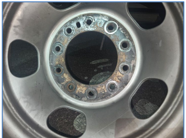
Top Photo – Taken immediately after discovering that eight of ten wheel studs were missing.
